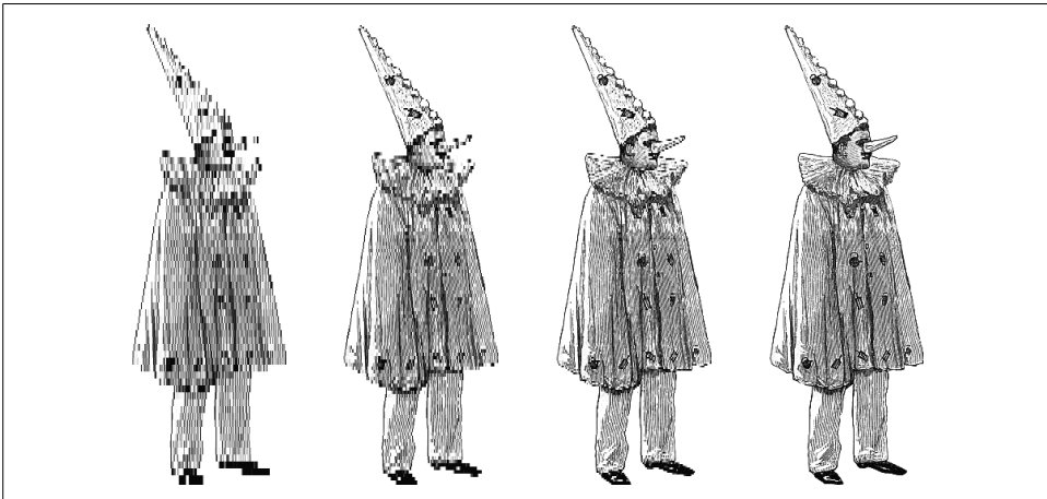
Figure 1-5. Interlacing provides a perceptual increase in download speeds by presenting a distribution of pixels as the image comes across the network
