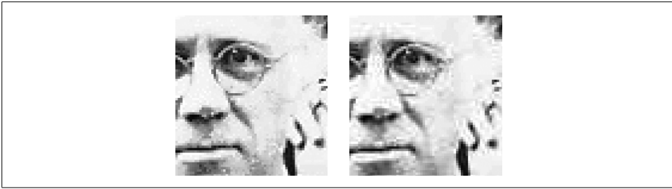
Figure 1-4. Repeated decoding and encoding of JPEGs can result in information loss
